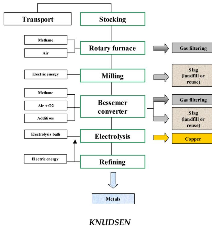
**Figure 4 – Model of pyrolysis process**
