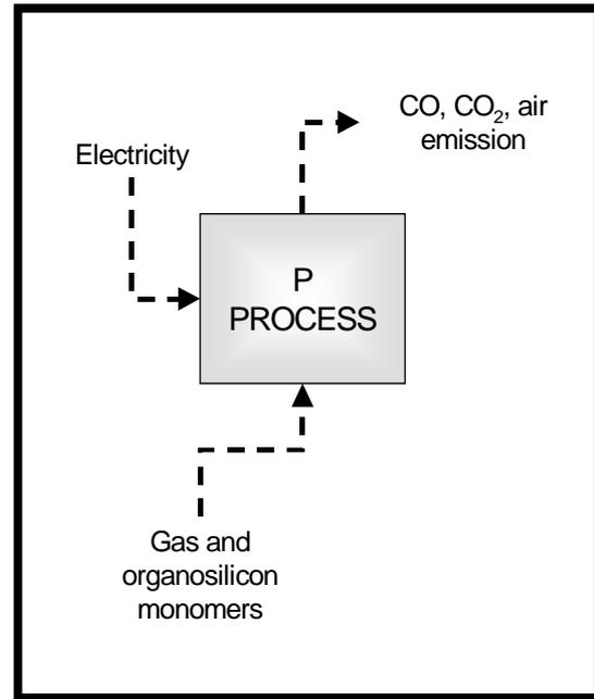
Figure 6 – System boundaries of P process
