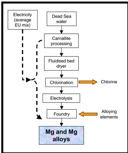
**Figure 3** – System boundaries of magnesium production
