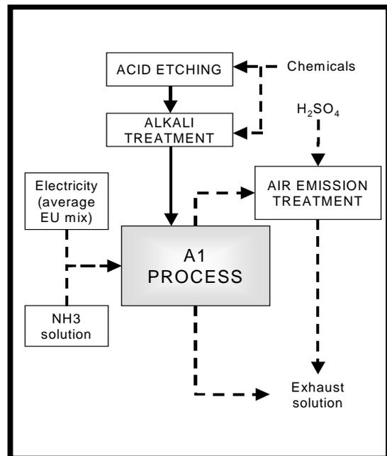
**Figure 4** – System boundaries of A1 process
