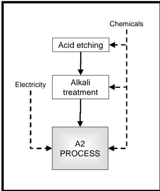
Figure 5 – System boundaries of A2 process
